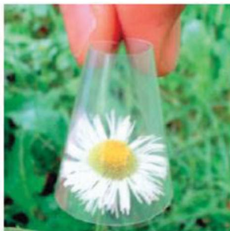
**Figure 14.** Flexibility and transparency of a  $65 \mu\text{m}$  thick BC-Acrylic resin nanocomposite sheet (60 wt% BC content).<sup>99</sup>
